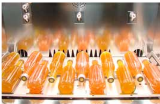
Light stability testing of beverages using the Atlas SUNTEST XXL+ FD
