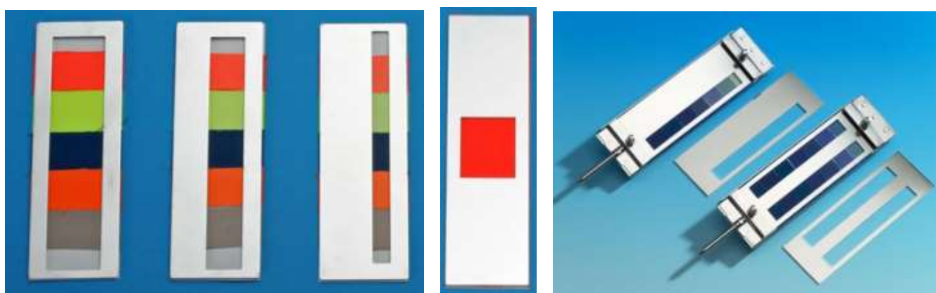
Figure 3: Left: ISO 105-B02 Exposure Method 2 cover masks. Center: AATCC cover mask. Right: ISO 105-B02 Exposure Method 3 (Marks & Spencer) cover masks.
