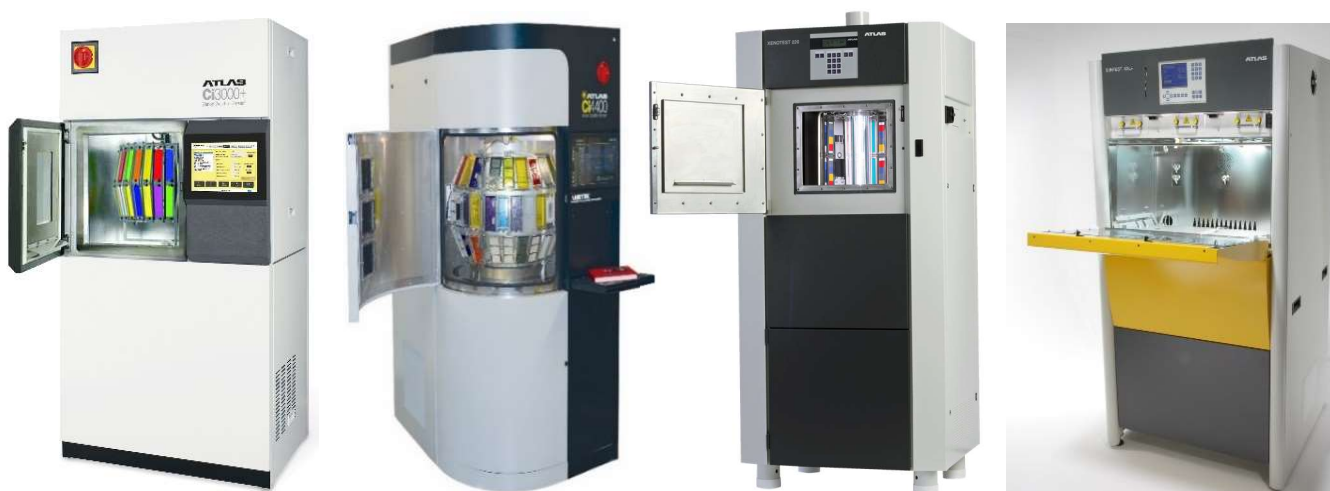
Figure 2 (left to right): Xenon-arc instruments meeting ISO 105-B10 and -B04. Rotating rack: Ci3000 Fade-Ometer®, Ci4400 Weather-Ometer®, Xenotest® 220. Flatbed: SUNTEST® XXL+.
